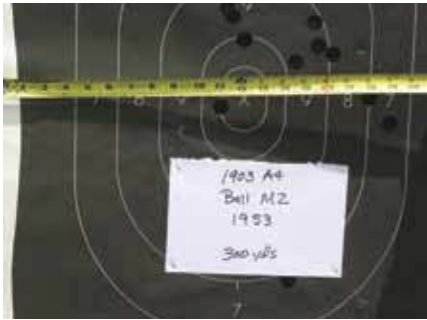
The original US Model 1903A4 shot poorly at 300 yards with original M2 ball issue ammunition dated 1953, with a 3-shot group of 17.5".
