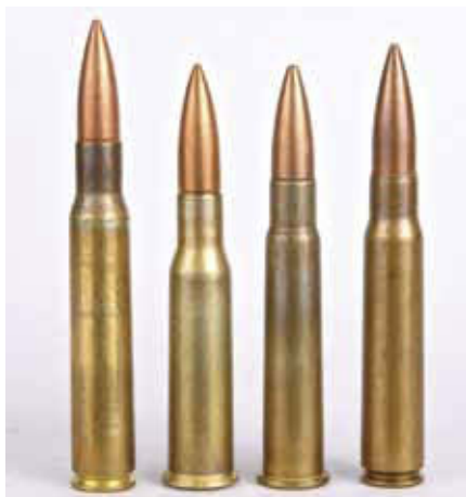
The original military issue ammunition from either World War II or the Korean War Duke and Dave Emary used for this informal test included (from left to right) US .30-06, USSR 7.62x54Rmm, British .303 and German 8x57mm Mauser.
