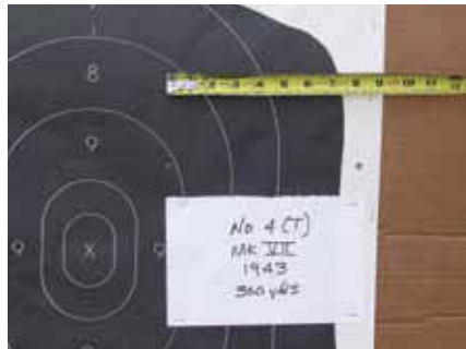
Even with mildly defective original .303 British military issue ammunition, the No.4, Mk I (T) sniper rifle performed fairly well out to 300 yards.
