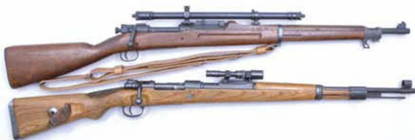
Duke's rebuilt US M1903 .30-06 is fitted with a 3X Leatherwood scope (top) and the original German K98k 8mm Mauser is fitted with Numrich reproduction 1.5X Zf41 scope.
