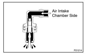
(3) Blow air into the air intake chamber side when lift up the inside valve, and check that there is a strong resistance to air flow.
