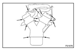
2. INSPECT HOSES, CONNECTIONS AND GASKETS Visually check for cracks, leaks or damage.
