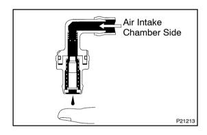
(2) Blow air into the air intake chamber side, and check that air passes through with difficulty.
