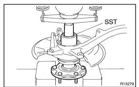
(b) Using SST and a press, install the axle hub to the steering knuckle.
