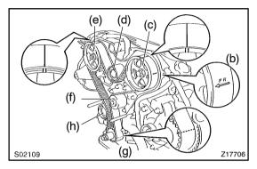
(c) Using SST, turn the camshaft pulley, align the timing marks of the timing pulley and No.3 timing belt cover. SST 09960-10010 (09962-01000, 09963-01000)
