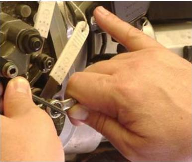
Now, don't be thinking this is a delicate maneuver. You're putting real power to the wrench, but, because you've choked up, and you're holding the pinky off the wrench, you're preventing yourself from putting a heavy fistful of twist on that locknut. If you put that pinky down, you're going to apply more force than you need. Experiment with the two grips by clamping an expendable bolt in a vice and wrenching a nut with pinky up and pinky down. There's a surprising difference.
