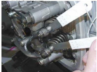
43. Clip your exhaust feelers to a cooling fin and insert the exhaust feelers (the 30's) into the exhaust valve assembly. Note: The exhaust valve assembly is at the 'front' the cylinder head near the exhaust headers.
