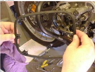
85. Put the rubber spark plug gasket back into/onto the cylinder head cover. You remembered to rotate this gasket so the plug indentations get virgin gasket, right? Ahhhh.
