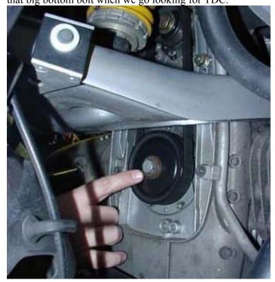
9. You'll find the engine timing hole on the 'Throttle grip' side of the engine. It's that little round slightly concave rubber plug behind the cylinder head, right up above the throttle body, just below the telelever hinge. Oh, for chrissakes, it's right HERE...
