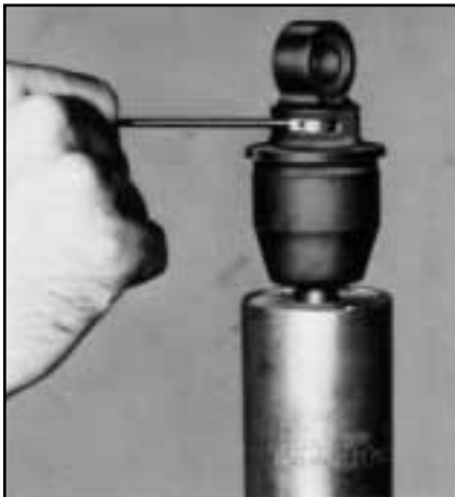
Figure 1. Move pin left to right to increase rebound forces (counter-clockwise).
