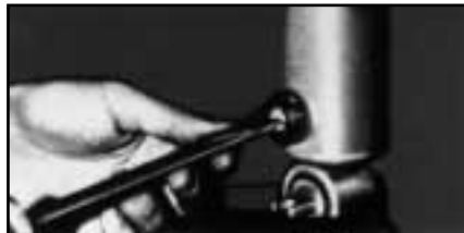
Figure 2. Turn screw from left to right to increase compression forces. (Clockwise)
