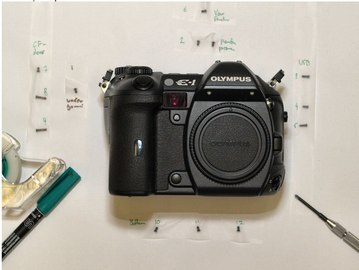
Keeping everything clean and tidy is essential. All screws are marked with the order they were removed and where they came from and scotched to the work-surface.
