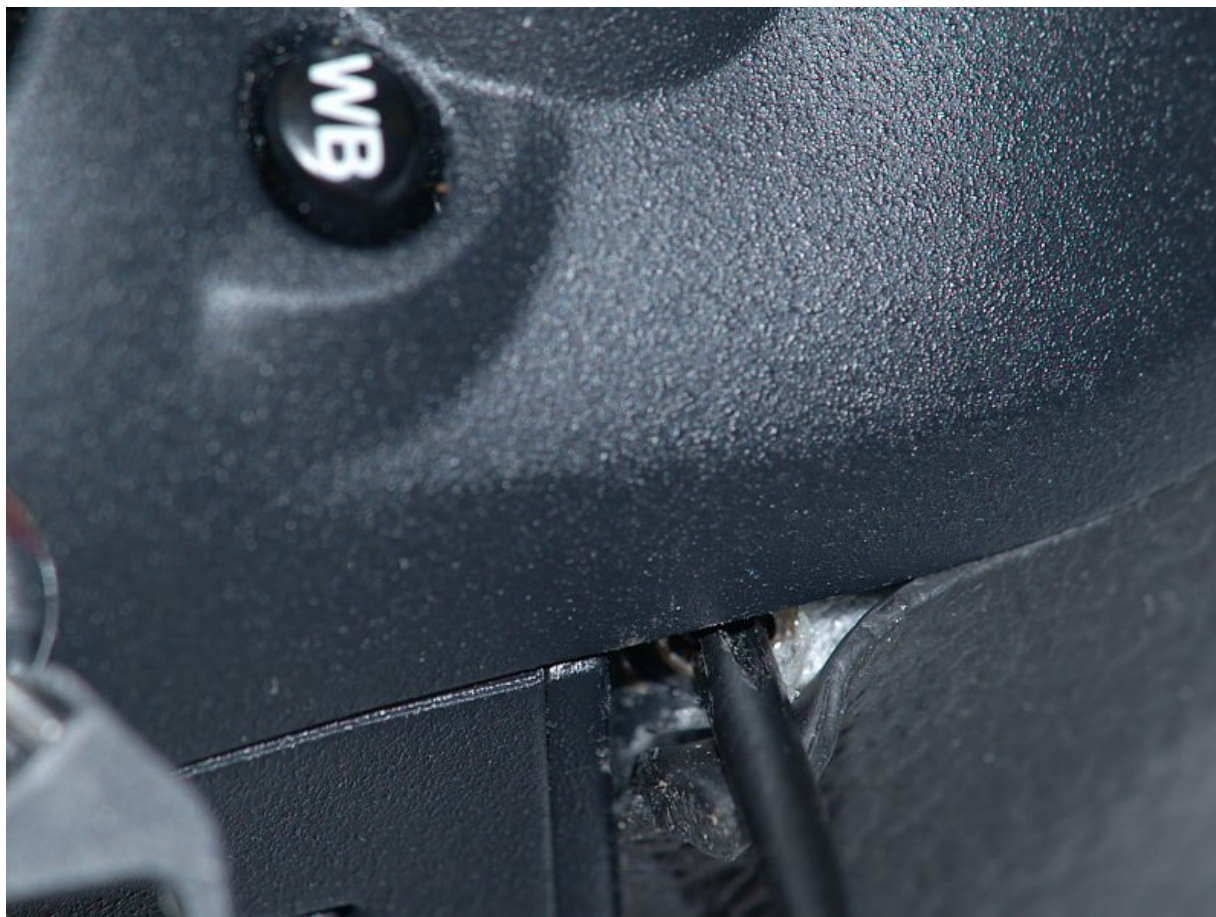
This is the only hidden screw - under the rubber.
