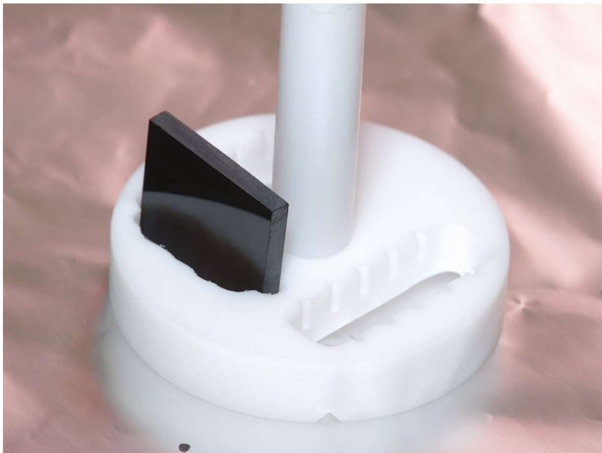
The new IR-pass filter (3 mm Schott RG780) is waiting in its ultrasonic cleaning fixture, ready to be put in place.
