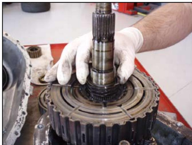
24. Install the cam with three (3) steel balls.
