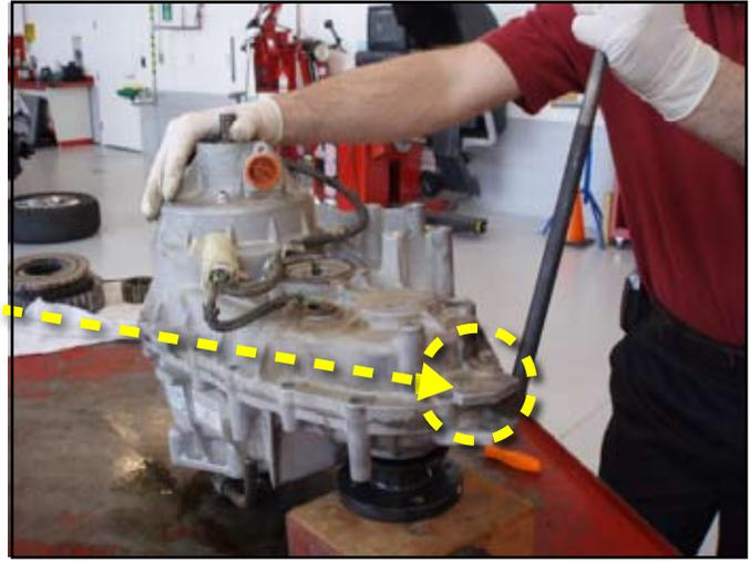
13. Carefully lift the case half straight upward to separate the case assembly.
