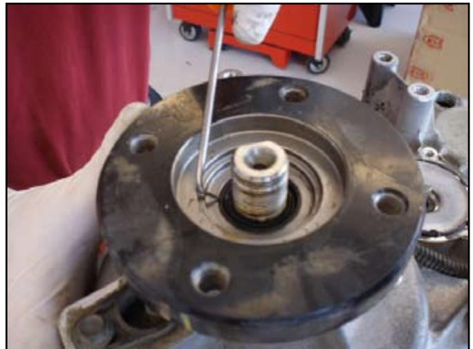
11. Remove the output shaft flange from the transfer case. Remove rear damper weight if necessary.
