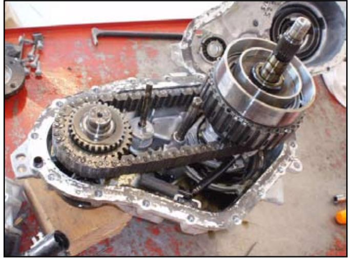
14. Remove the output shaft bearing.
