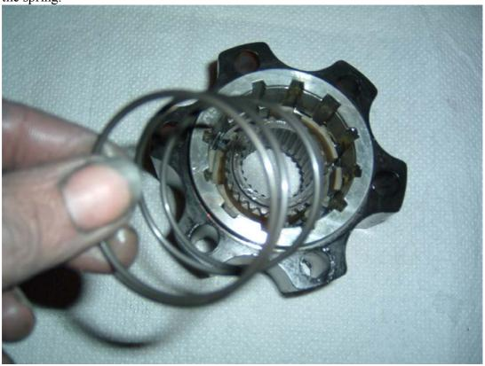
Replace the lockup ring. Some of you will have one which is flat on both sides, but mine have a shoulder which means it will only go in one way round. The shoulder goes to the outside.
