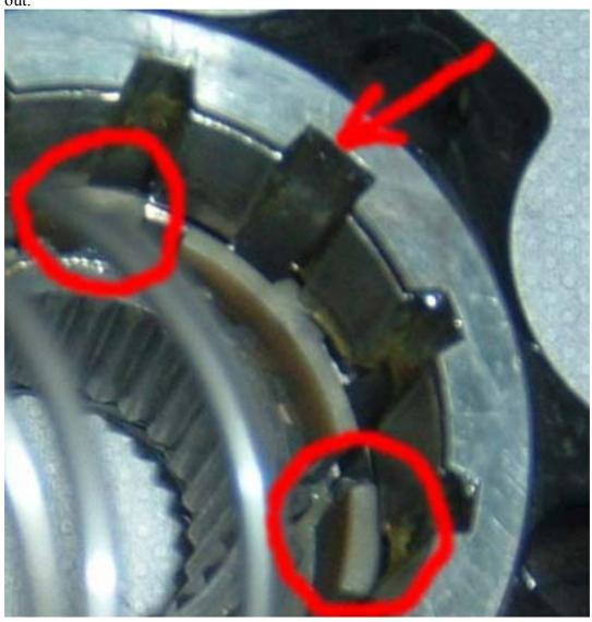
The inner gear bush is held together by two clips which can be prised apart and the
