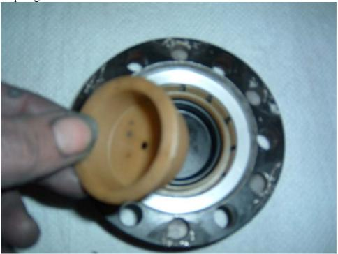
Using a small flat screwdriver, lever out the locking tabs on the retaining ring and remove it
