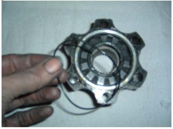
Turn the whole assembly the other way up, smear the inside with grease and install
