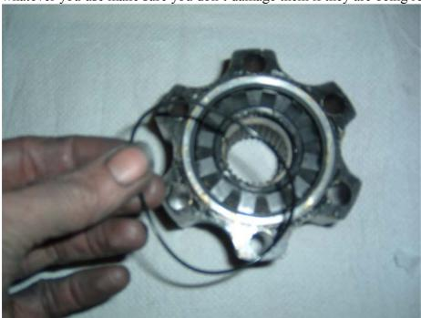
Remove the front lockring with a screwdriver, starting at one end and working round, this is under tension so it will try to fly out.
