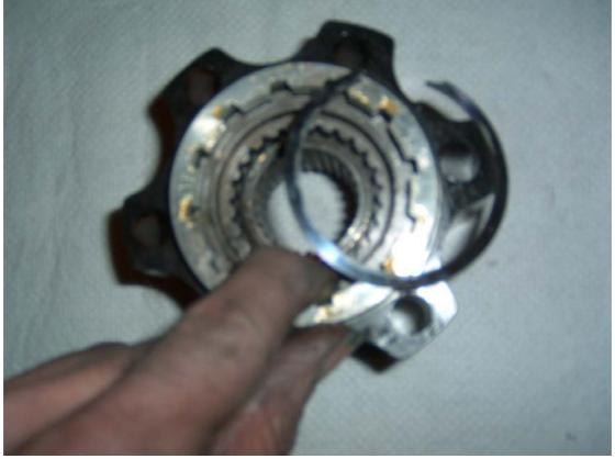
Lift out the lock up ring and the spring underneath.
