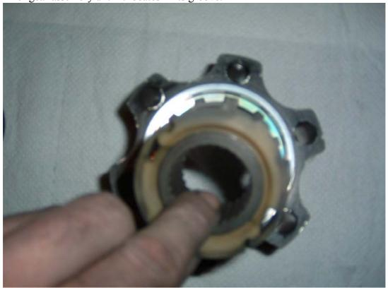
The rear lockring can now be replaced into its groove. You will notice one end of this has a cutaway, this should be located in the squared guide to allow easy removal.
