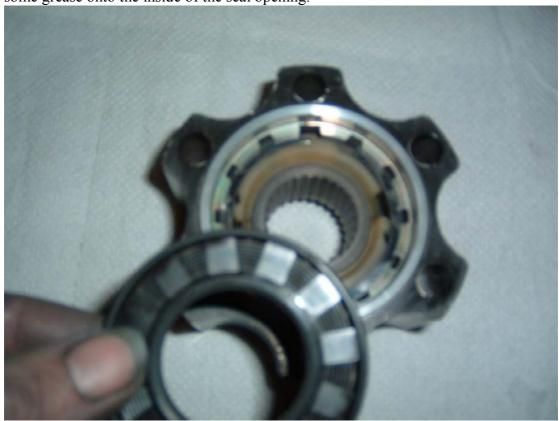
Replace the rear o-ring, greasing both the location grove and the o-ring when its in place.
