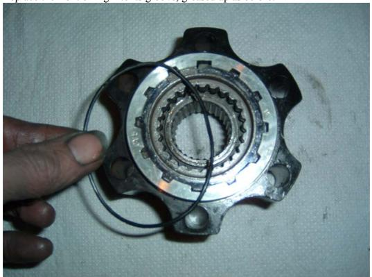
Before replacing the assemblies onto the vehicle, smear some grease on the splined interior of the inner gear and the shim.
