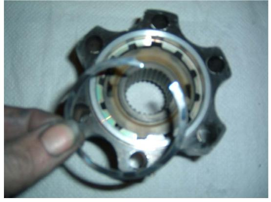
The rear seal can now be pushed into place. The flat side goes on the inside. Smear some grease onto the inside of the seal opening.
