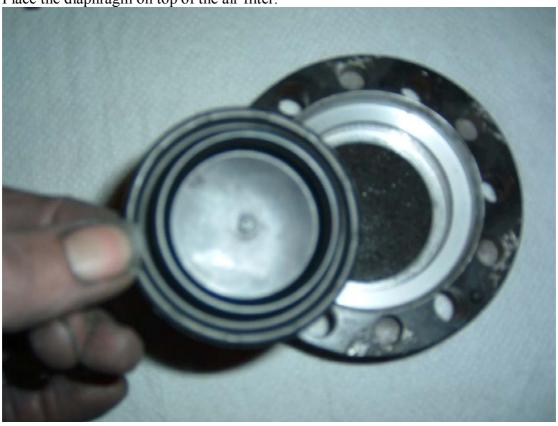
Push the retaining ring into place and using a screwdriver ensure the tabs are secured.
