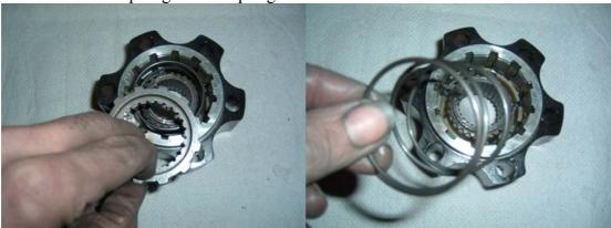
Whilst applying some pressure from underneath, use a screwdriver to prise the locking tabs on the plastic inner gear bush out of their location groove. There are two each side of the squared guides. It's a tight fit and requires a bit of pressure to get it out.
