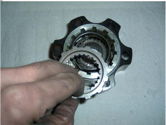
Now comes a fiddley bit. Holding the lockup ring down with one hand, use a screwdriver to ensure the spring is central, once it is, push down harder and engage the lockup ring with the inner gear. Still holding the lockup ring in its engaged position the front lockring must be located in its groove. Again the cutout in the end should be located at the squared guide.
