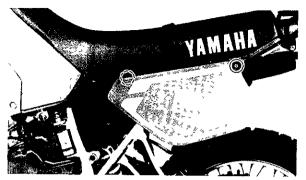
b. Remove the stopper bolt and then remove the radiator cap.
